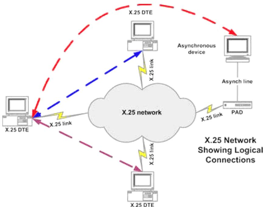
The X.25 standard corresponds in functionality to the first three layers of the Open Systems Interconnection (OSI) reference model for networking. Specifically, X.25 defines the following:
